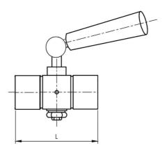
Gauge Cocks provide an econimical and simple way to shut off the flow to a pressure instrument. Thereby, allowing the instrument to be isolated from the pressure media or removed from service. These are often used in conjuntion with a U or O syphon to suit.
