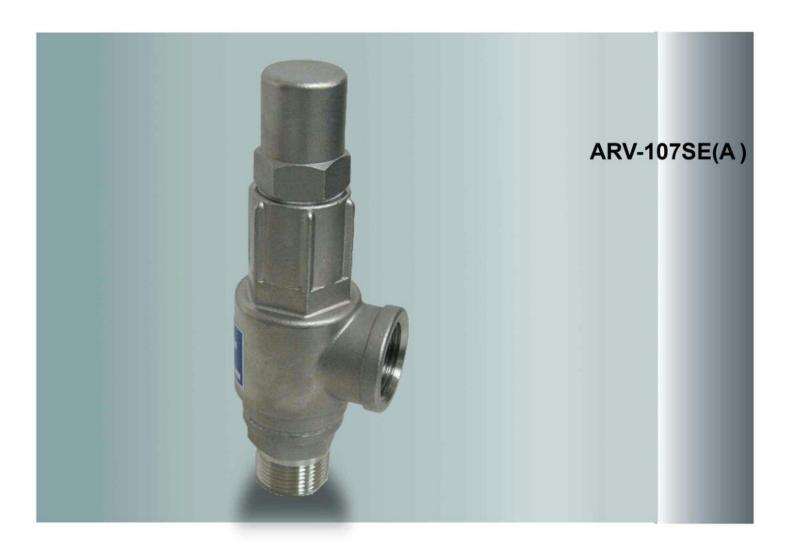
The stainless steel body components are investment cast to give fine finishing and structure strength. The disc is freely pivoted by the spindle and its linear movement is closely guided to ensure correct alignment with the seat for tight sealing. The displacement of disc is designed to provide maximum discharge capability. The valves are suitable for gas, steam and liquid application. Every valve is set at designed working pressure and tested in the factory before packing.
