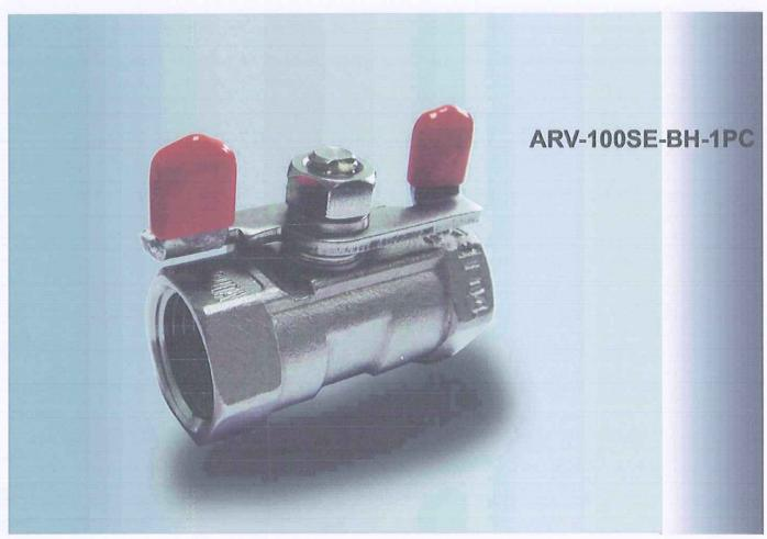
The stainless steel body is a one piece compact design and is investment cast to provide high quality finishing and structural strength. It is also less prone to leak owing to it one piece body. The ball and seats are of high finishing quality. This contributes to good sealing and low operating torque. This product is suitable for general and industrial applications.
