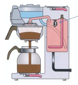
OLV-5T is installed at the top of water heating tank to prevent overflow.
