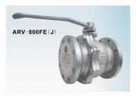
Aria full bore ball valve design offers a smooth and subulence-free flow of media. The stainless steel ball is housed in a rigid and rugged two pieces cast iron body. The PTEE seats are precisely machined and hold the ball firmly in the housing and at the same time provides excellent sealing. A blown-out proof stainless steel stem is used to open or shut the valve. This operation can be done manually with a lever or gear, electric actuator, or previously caused to the proof of the proof of
