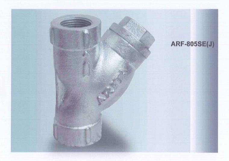
Arita Cast Iron Y-Strainer is a device which provides a mean to remove debris from a flowing fluid in a pipeline. A perforated screen or mesh is used to trap the debris in the strainer chamber. The strainer chamber is designed with a plug or cover that can be easily removed for maintenance purposes. The Y-Strainer can be installed either in horizontal or vertical down position and must be always before the valve or equipment.
